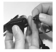
6. Plug the finger sensor into the pod.
