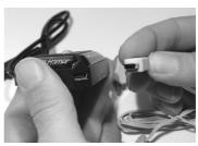
An optional ear sensor may be plugged into the pod instead of the finger sensor.
