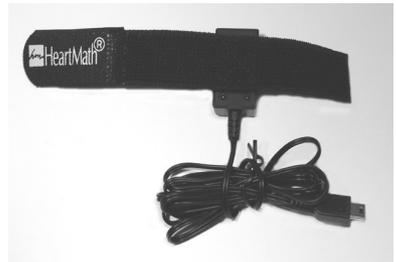
5. Place the tip of your finger on the finger sensor and then gently wrap the strap--starting with the short end--around your finger to secure the sensor to your finger. Your finger should feel snug between the sensor and strap but you should be able to slide your finger in and out easily.
