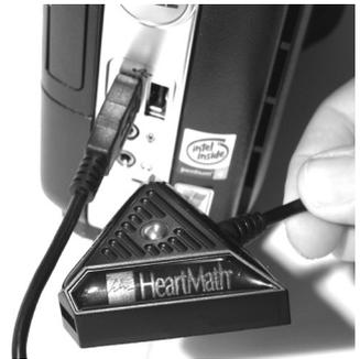
2. If the pod cable cannot conveniently reach a USB port on your computer, unwrap the USB extension cable and connect the male end of the cable to a USB port on your computer or USB hub.
